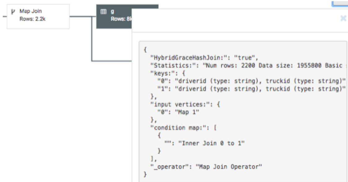
Figure 6.6. Details of a Map Join Node
