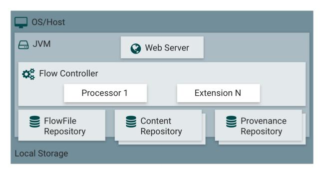
NiFi executes within a JVM on a host operating system. The primary components of NiFi on the JVM are as follows:
