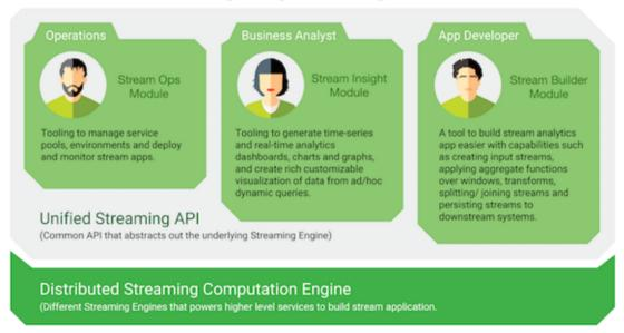
You can think of Streaming Analytics Manager as an application that operates on top of a streaming engine (a "gray box") that allows you build stream apps faster on top of your selected streaming substrate. The unified streaming API provides the abstraction that allows you to plug in different streaming engines.
