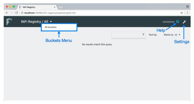
The Buckets menu is available at the top left of the screen. It allows the user to display flows based on which bucket they are contained in. On the top right of the screen is the Settings button
