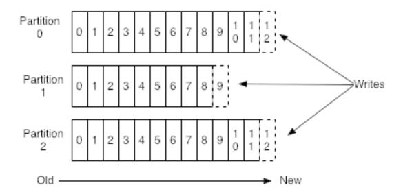
Kafka appends new messages to a partition in an ordered, immutable sequence. Each message in a topic is assigned a sequential number that uniquely identifies the message within a partition. This number is called an offset, and is represented in the diagram by numbers within each cell (such as 0 through 12 in partition 0).
