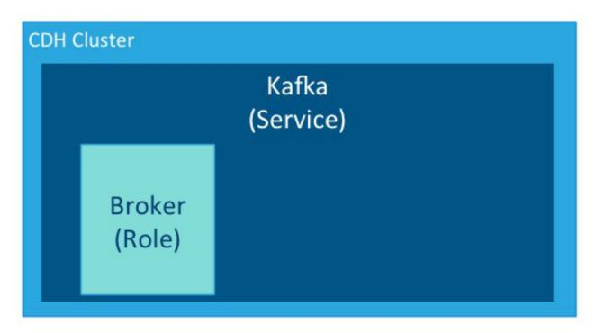
An *instance* is a deployed and configured software component. A cluster can include multiple roles and multiple instances of the same role. A *service instance* might be Kafka-1. Kafka-1 might host the *role instances* Broker-1, Broker-2, and Broker-3.
